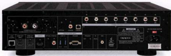
ABOVE: Inputs include two HDMI (main and 'audio only'), coax/optical S/PDIF, Ethernet, USB-B (for PCs) and two USB-A 3.0 sockets for external HDDs. There are two HDMI outs, with 7.1 channel plus stereo RCA and balanced XLR analogue audio outs
